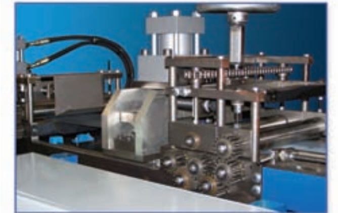
Flying Hydraulic Pre-Punch and Pre-Cutoff System.
