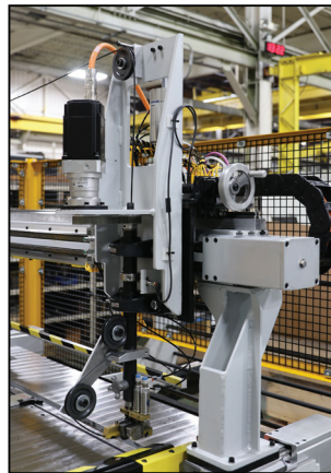
Enhanced z-axis positioning with hand wheel and counter for better height control and faster changeovers
