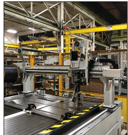
Rigid construction of bridge mounted to linear rails and driven on both sides.
